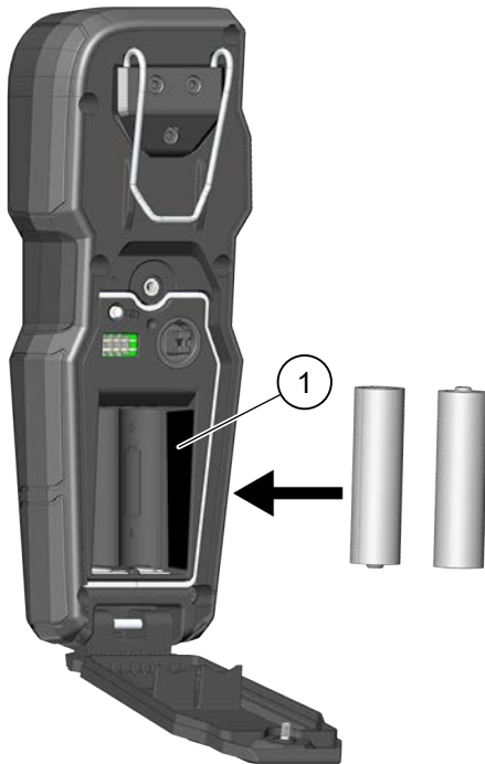
Figure 1. Installing Remote Control Batteries
