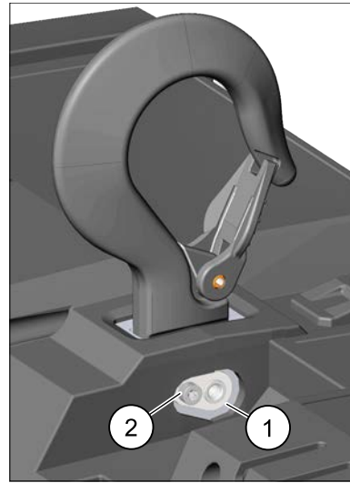
Figure 7. Suspension Pin Retainer/Retainer Screw
